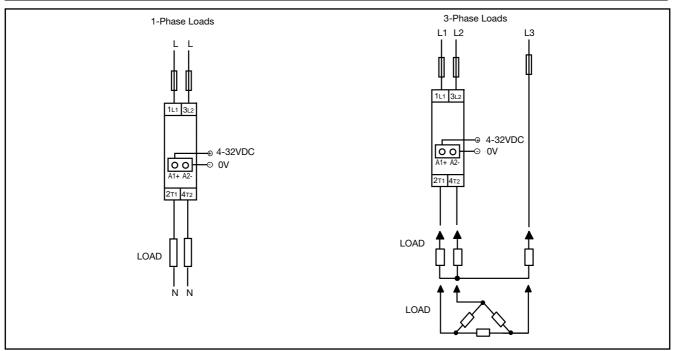
Note: Application of control voltage to terminals A1 - A2 will activate both poles simultaneously.
