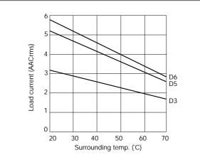
Derating curve is used for finding max. load current at an elevated ambient temperature. The 3 lines in the graph represent the 3 nominal current ratings of the RP1 series (RP1...D3/D5/D6).
