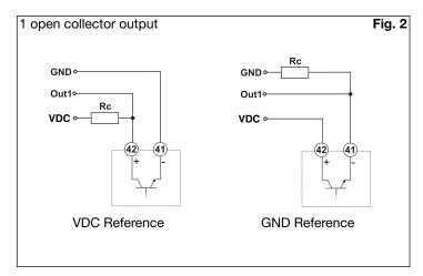
The load resistances (RC) must be designed so that the close contact current is lower than 100mA; the VDC voltage must be lower than or equal to 30VDC.
