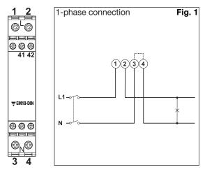
**NOTE:** The 3 and 4 terminals, in the instrument, are wired together
