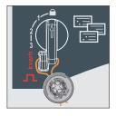
Lock of programming with seal. Selection of up to 4 main pages (programmable by the user).
